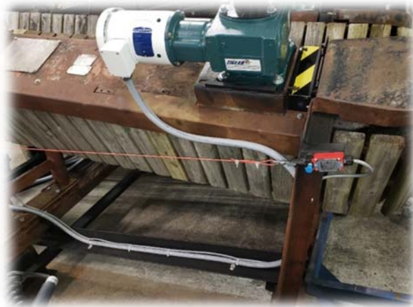
Rope pull on V-Conveyor – 2 places – each side of the V-conveyor
