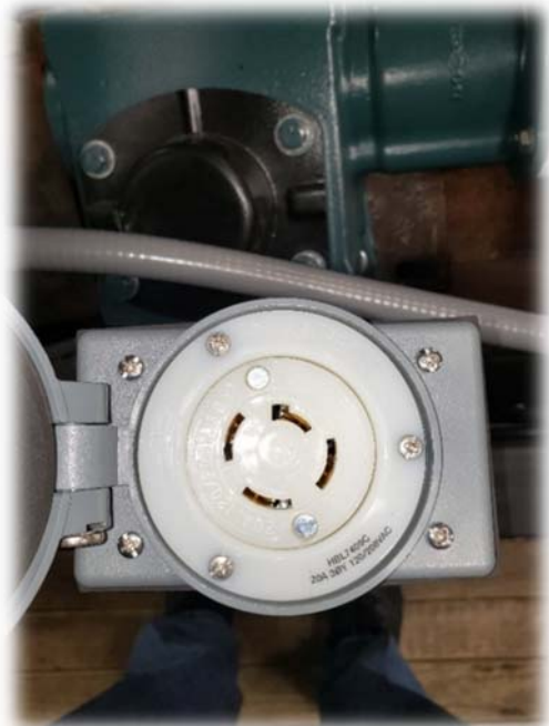
Stunner wand plug receptacle located on each end of the platform.
