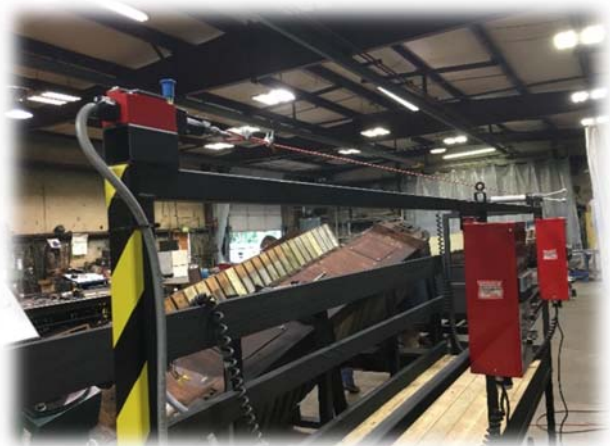
Rope pull on V-Conveyor – 2 places – each side of the V-conveyor
